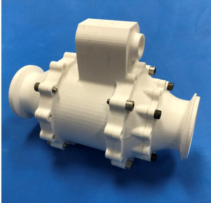
The option to print prototypes in durable real engineering-grade ABS is another benefit of using the METHOD X. However, Colby is excited about the possibilities offered by MakerBot's rapidly expanding materials portfolio, in particular MakerBot Nylon Carbon Fiber.
