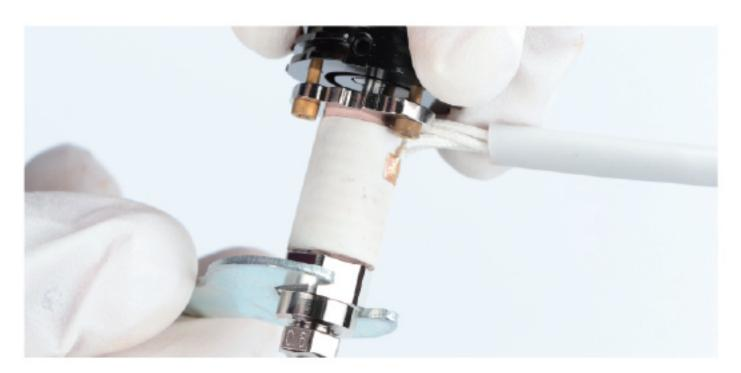
3. Screw the copper plated adapter nut with the H10 open - ended wrench, and stick the hexagon side of the nut to the bottom of the heatblock (The two sides should be fit tightly where the red arrow points below).
