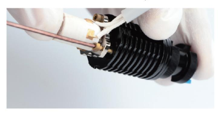
Tighten the M3\*6 screw on the heatsink, and push the groove of the plug core against the capillary.
