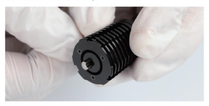
4. Insert the capillary tube on the heatblock to the central hole at the bottom of the heatsink, and the three holes on the heatblock should be aligned with the three supporting tubes on the heatsink.
