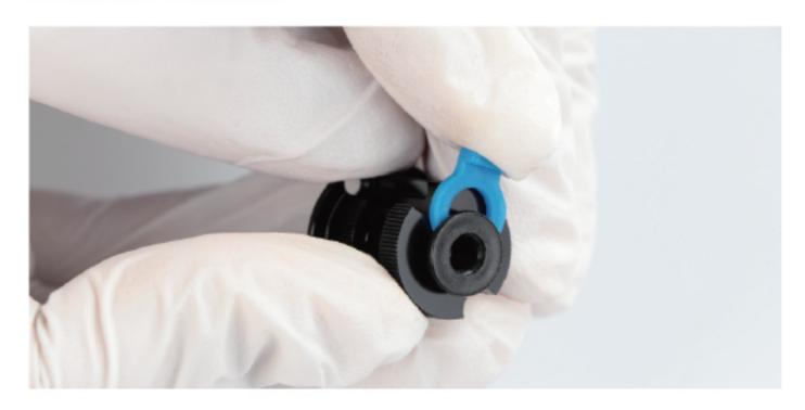
Install the adapter on the heatsink using the M2.5\*5 screws.
