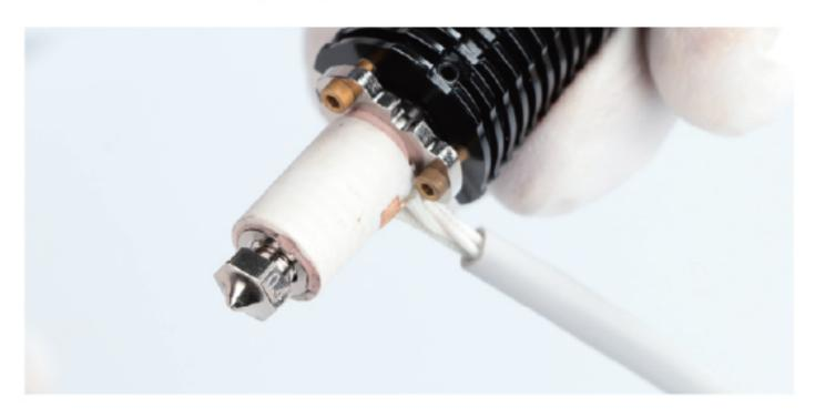
Install the nozzle on the heatblock in hot tightening way.
