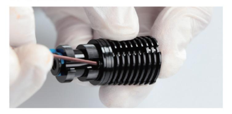
Insert the plug core into the large hole at the bottom of the heatsink, and gently hold the heatsink with a M3\*6 head screw (the groove faces the central hole).
