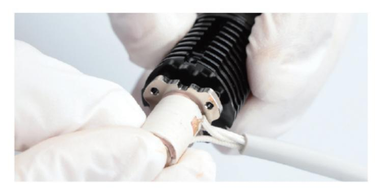
5. Align the three supporting tubes at the bottom of the assembled heatsink with the three round holes on the heatblock (the direction of the wire on the heatblock should be staggered with the position of the head screw on the heatsink), and screw the titanium alloy screws of M1.6\*12. (The gap between the heatblock and the heatsink is about 2.5mm).
