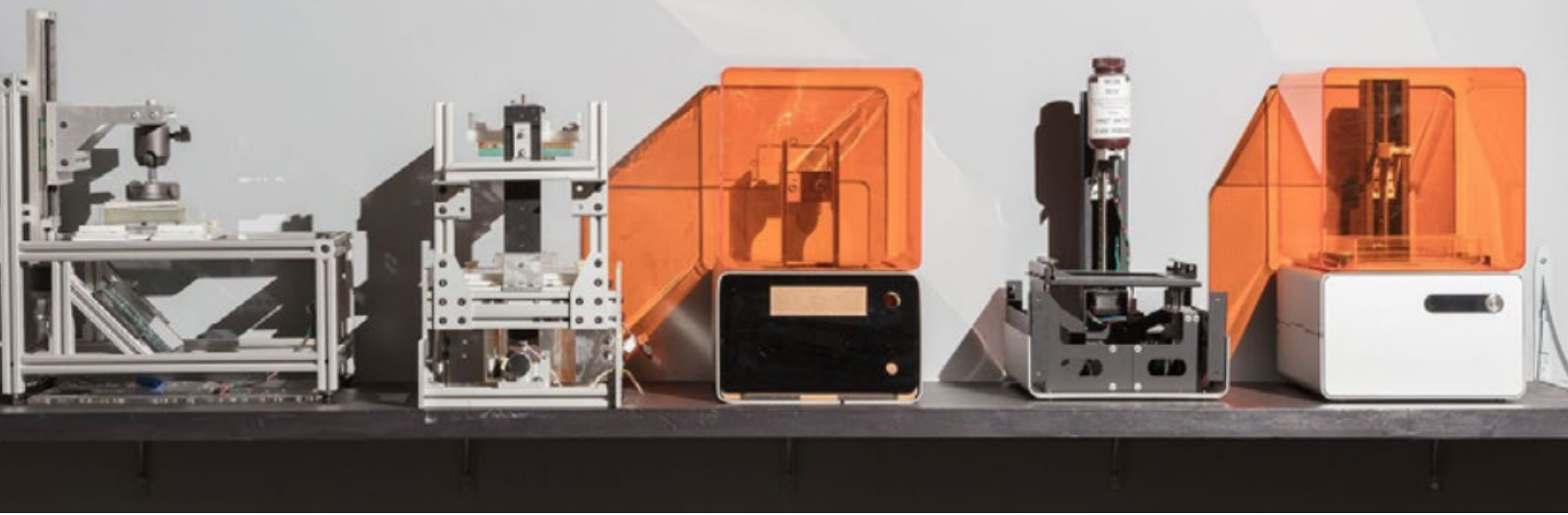
Prototypes of the Form 1, the first desktop SLA 3D printer.
