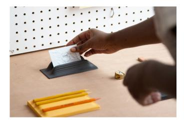
This ridged shape was then vacuum formed using the FormBox to create a set of molds. By filling these molds with a casting material called Jesmonite, Charlie was able to make a set of objects in different colours designated by various pigments.
