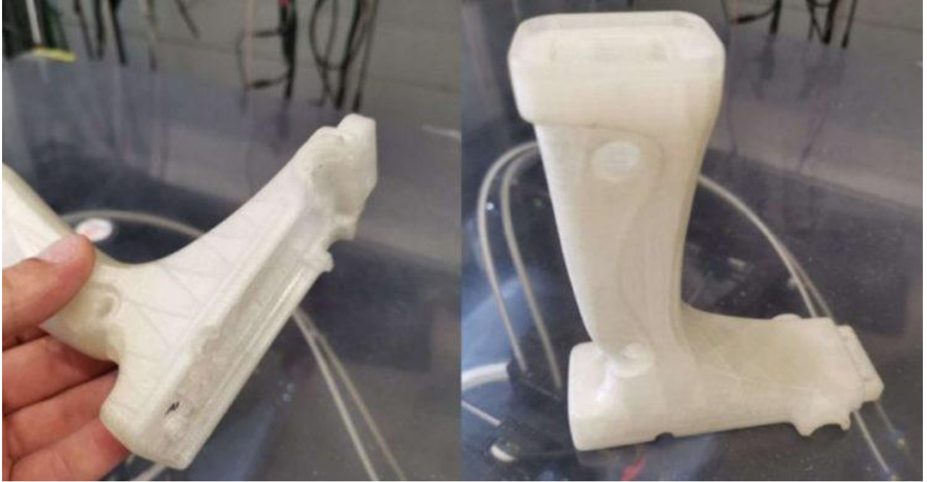
Antenna after printing on Raise3D Pro2 Plus
