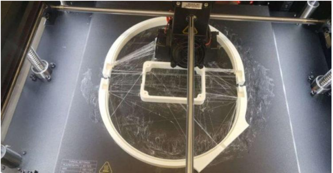
MRI coil printing on Raise3D Pro2 Plus
