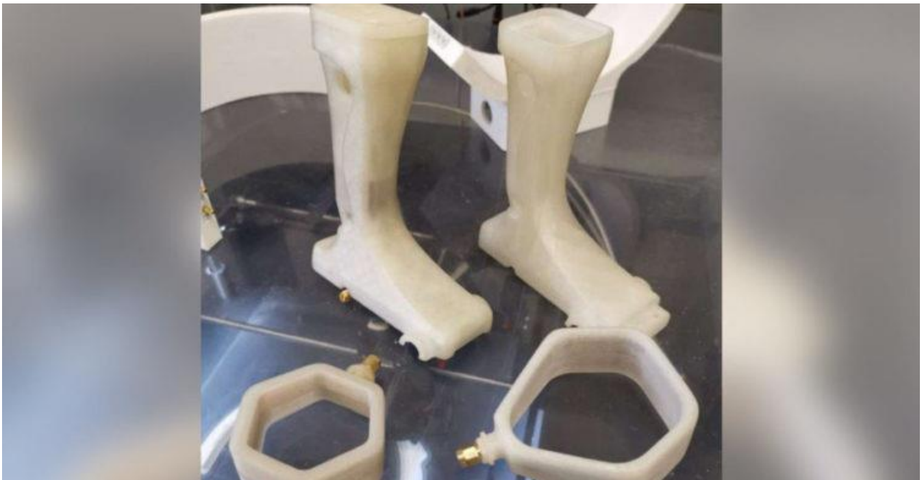
Antenna after printing on Raise3D Pro2 Plus
