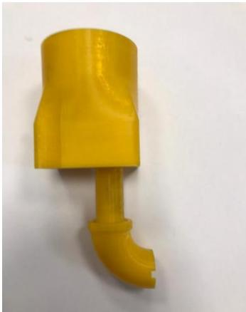
Another example is a suction system Sonmak printed to remove dust from their machine, to prevent the dust from spreading into the environment.
