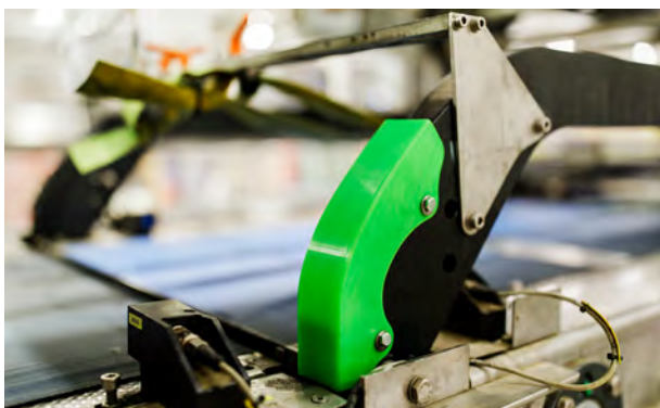
3D printed functional replacement parts can be created without stock
