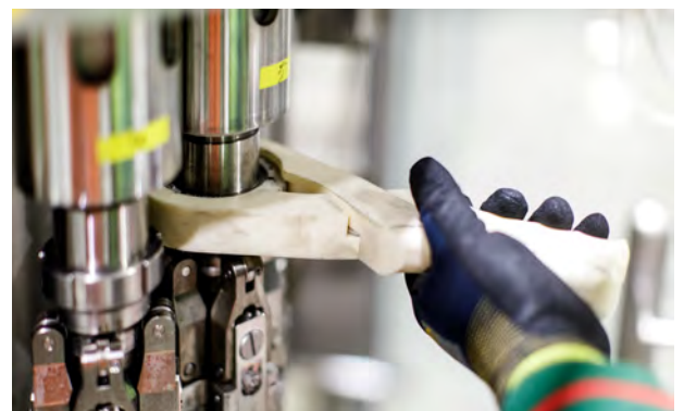
3D printed tools make maintenance easier and less time consuming
