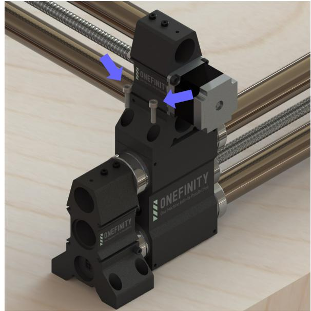
**Step 6:** Fasten the back of the X-Rail to the Y-Axis using the remaining four (4) X-Rail Mounting Screws (Green Arrows)
