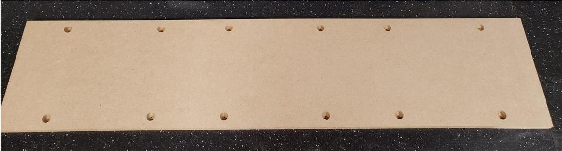
**Step 6:** Using a 1/16" Drill Bit, drill through holes in the centre of the counter bored holes.
