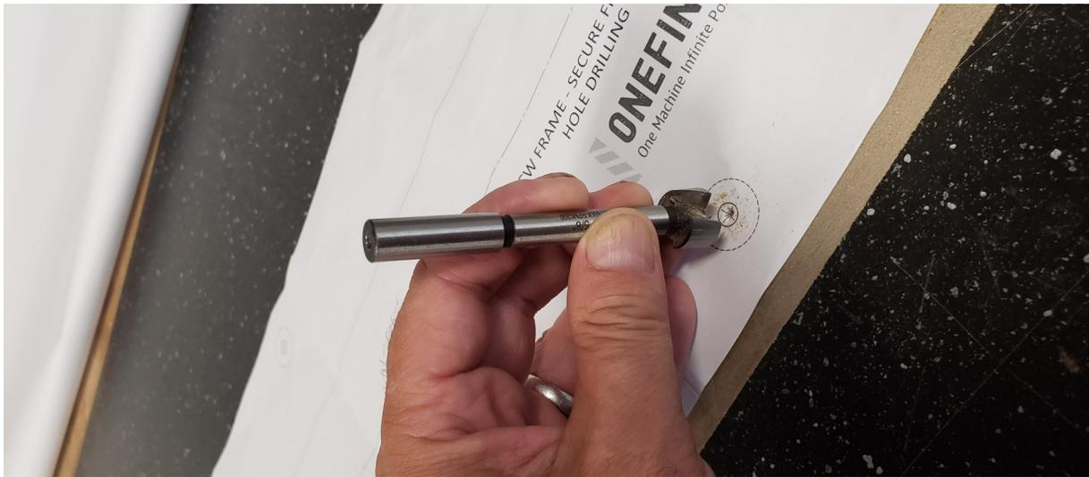
**Step 4:** Insert your Forstner Bit into your drill and counter bore holes in the locations you centre punch in step 3. **Important Note:** Counter bore to a depth of 3/8"
