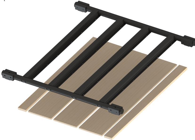
**Step 2:** Ensure the wasteboard is flush with the front of QCW Frame Tube and secure your wasteboard using the supplied screws. **Very Important Note:** Set the torque on your drill to low and finish tightening the screws with a hand screw driver. If your drill torque is set too high the screws may strip!
