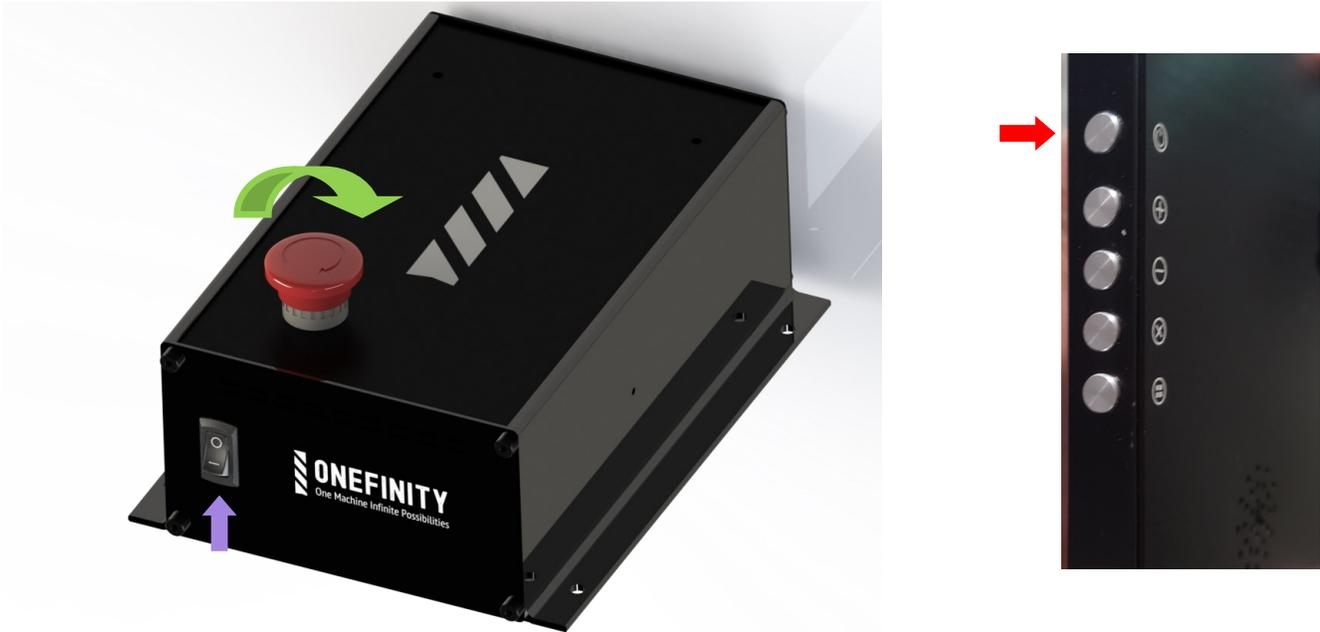
**Step 13:** We will now jog the Y-Axis so we can finish fastening the Y-Rails to the table. First ensure you are using metric units (Blue Arrow). If metric is not selected, tap the drop down arrow and select metric. Next, hit to 100 button (Green Arrow). This sets the Jogging distance to 100mm.
