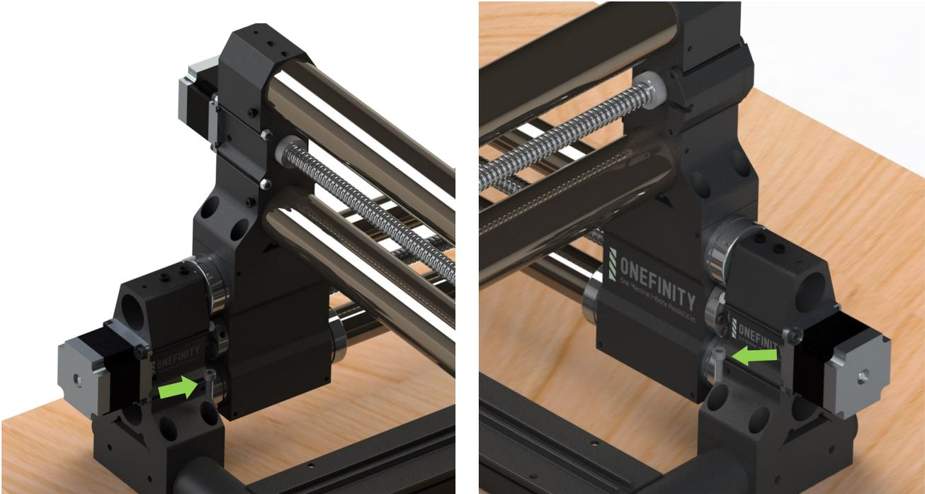
**Step 17:** We will now jog the Y-Axis to bring the X-Rail back to the front of the machine. Tap the Y- button (Green Arrow) 8 times. When finished the Y position should read 0mm (Blue Arrow)
