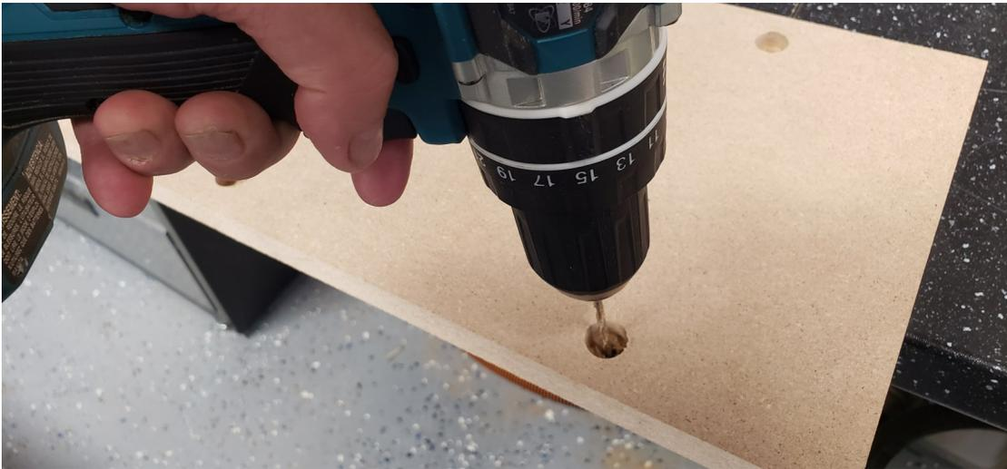
**Step 7:** Flip over the Wasteboard strip so the counter bore holes are facing down. With the wasteboard strip flipped over, drill open the 1/16" holes you drilled in step 6 using a 1/4" Drill Bit.
