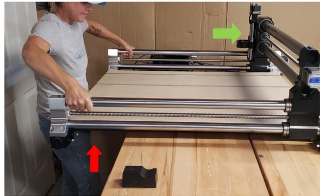
**Step 3:** Flip up your Ofinity CNC and place the QCW Stand under the Frame Tube.
