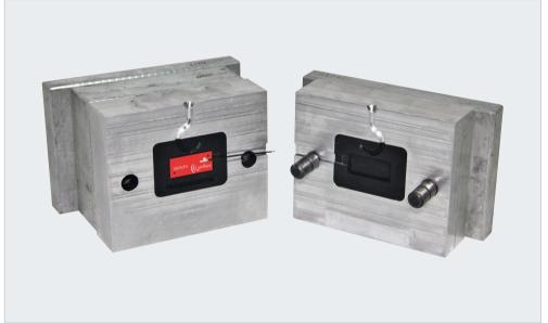
Rigid resin designed for tooling and molding applications owing to its high stiffness and high temperature resistance withstanding up to 230°C
