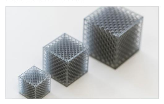
One-part elastomeric material formulated to have firm compression properties with quick rebound performance to match soft rubber like materials. Flexibility, high resilience and good energy return make this material ideal for gasketing, sealing and anatomical model type applications.
