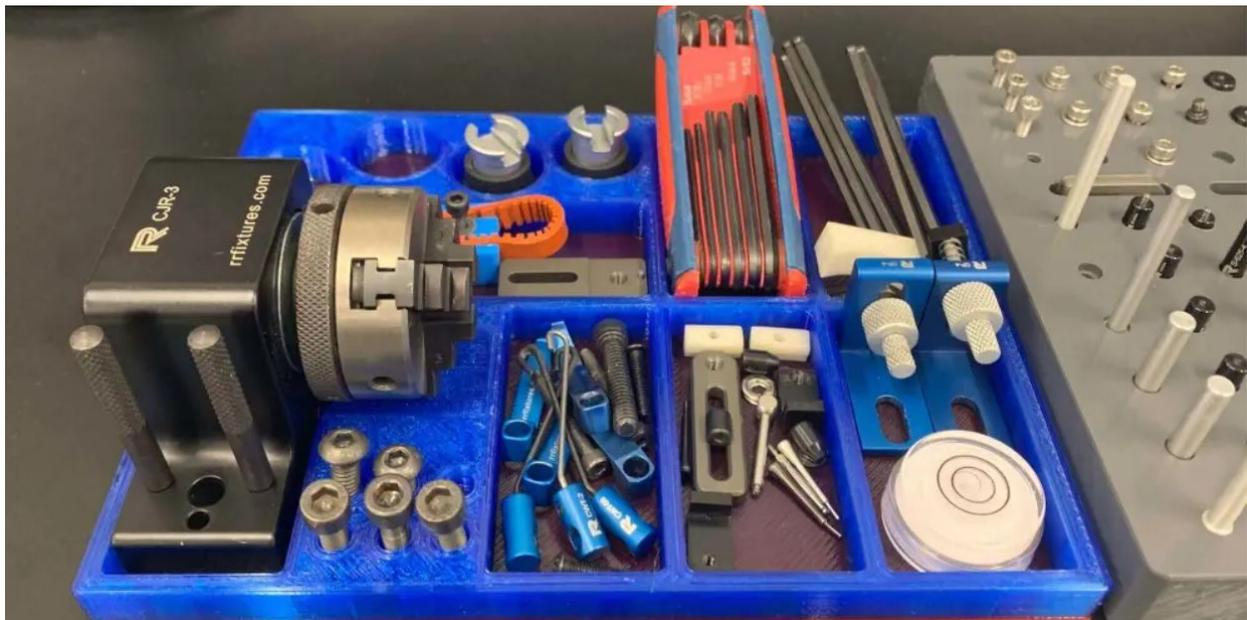
*Custom 3D printed tool storage, demonstrating the lean manufacturing 'poka yoke' principle*
