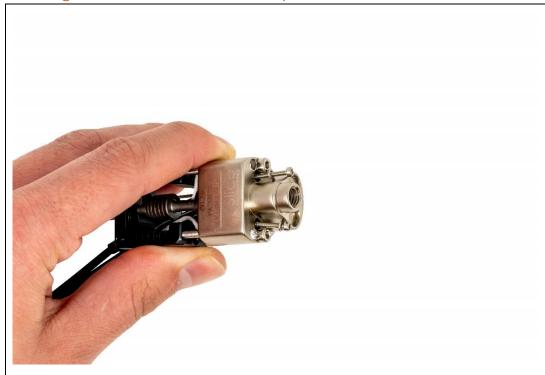
Insert the M1.6 x 0.35 Screw and Serrated Safety Washer assembly into the bottom of the Hot Block.
