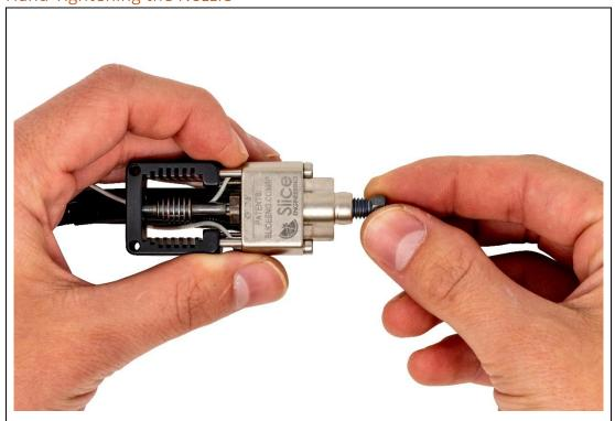
Manually screw the Nozzle onto the Hot Block in a clockwise direction.
