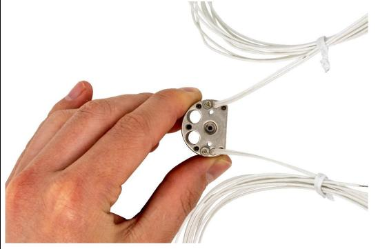
Attaching Retaining Screws for Temperature Sensor(s) (Part 2)
