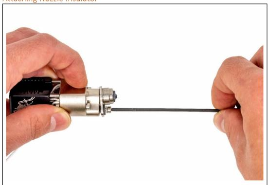
Tighten the screw with the 2 mm hex key until the Nozzle Insulator is parallel to the bottom surface of the Hot Block.
