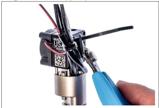
Use a pair of cutters to cut the excess length from the Panduit Cable Tie.
