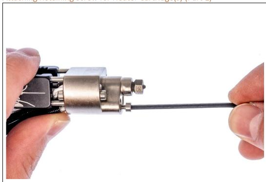
Thread the M2.5 x 0.45 x 8 mm **Retaining Screw into** the remaining tapped hole on the bottom of the Hot Block.
