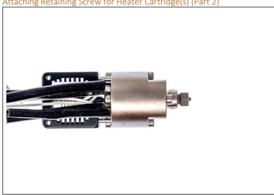
The M2.5 x 0.45 x 8 mm Retaining Screw head should be flush with the bottom of the Hot Block.
