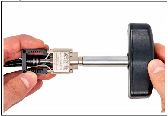
While either holding the hotend in your hands or a vise, use a 1.5 Nm Torque Wrench to fully tighten the Nozzle onto the Hot Block by rotating clockwise with the Torque Wrench until it clicks.
