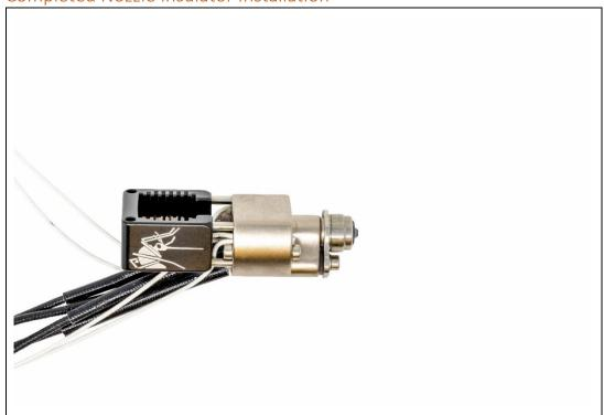
The Nozzle Insulator is parallel to the bottom of the Hot Block.
