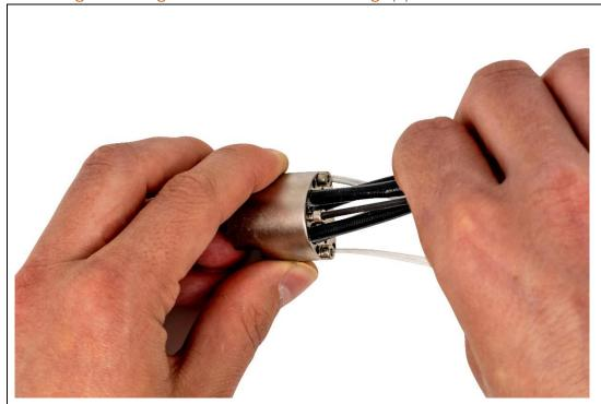
Thread the Retaining Screw into the Hot Block into the previously defined tapped hole.
