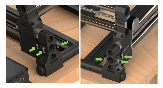
**Step 19:** Repeat steps 14 and 15 to jog the Y-Axis until the X-Rail is to the back of the machine again. Finish fastening the Y-Rails to the QCW Frame using the remaining three (3) Y-Rail Mounting Screws per side (Green Arrows).
