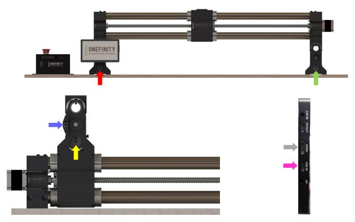
**Step 12:** It's now time to power up your machine. Start by twisting the Emergency Stop Button clockwise to release it to the "ON" position (Green Arrow). Next make sure your display is plugged into the Controller and a wall outlet and turn on the Touch Display by pushing the ON button (Red Arrow). Finally, flip the switch to the ON position (Purple Arrow).
