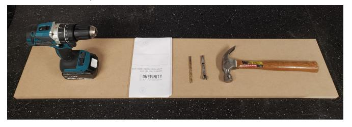
**Step 2:** Lay the Drilling Template on top of the MDF Wasteboard strips. If you wish, you can use painters tape to keep it in place.
