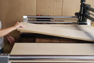
QCW Frame Secure from Beneath: Changing your wasteboard with the Onefinity CNC installed.
