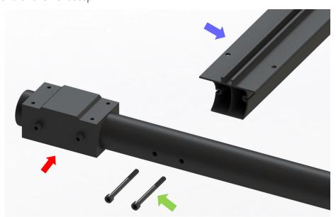
**Step 2:** Attach the rest of the T-Track Extrusions to the QCW Frame Tube Assemblies using the remaining QCW Frame Assembly Bolts. **Note:** To make the assembly process easier, wait until you have all the T-Track Extrusions attached before fully tightening the QCW Frame Assembly Bolts.
