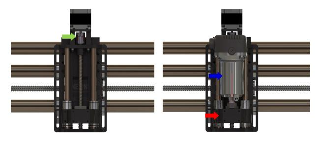
**Step 2:** Slide the Router all the way down in the Spindle Mount. Tighten the Spindle Mount Screws (Green Arrows)
