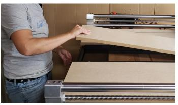
**Step 2:** Using your drill with the Robertson bit installed, secure the front of the Wasteboard Piece using two of the supplied Wasteboard screws. **Very Important Note:** Set the torque on your drill to low (we will finish tightening the screws with a hand screw driver later). If your drill torque is set too high the screws may strip!
