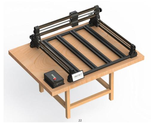
**Step 16:** After moving the X-Axis all the way to the back, fasten the back of the Y-Rails to your QCW Frame using only one (1) Y-Rail Mounting Screw per side (Green Arrow).
