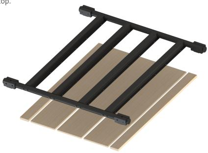
**Step 2:** Ensure the wasteboard is flush with the front of QCW Frame Tube and secure your wasteboard using the suppled screws. **Very Important Note:** Set the torque on your drill to low and finish tightening the screws with a hand screw driver. If your drill torque is set too high the screws may strip!
