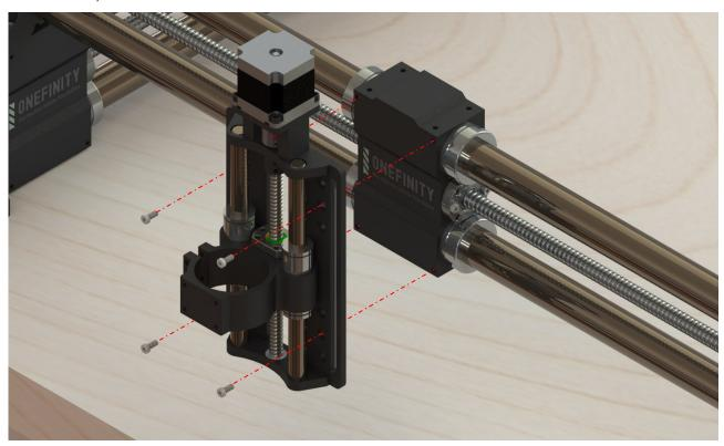
**Step 21:** Square the Z-Slider to your table then tighten the Z-Slider Mounting Screws. Next, plug the Z-Sliders stepper motor into the Curly Cable. **Congratulations, you have finished assembling your new Onefinity CNC Machine!**
