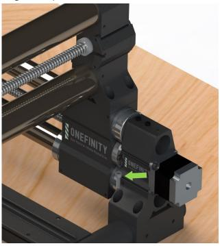
**Step 17:** We will now jog the Y-Axis to bring the X-Rail back to the front of the machine. Tap the Y- button (Green Arrow) 8 times. When finished the Y position should read Omm (Blue Arrow)
