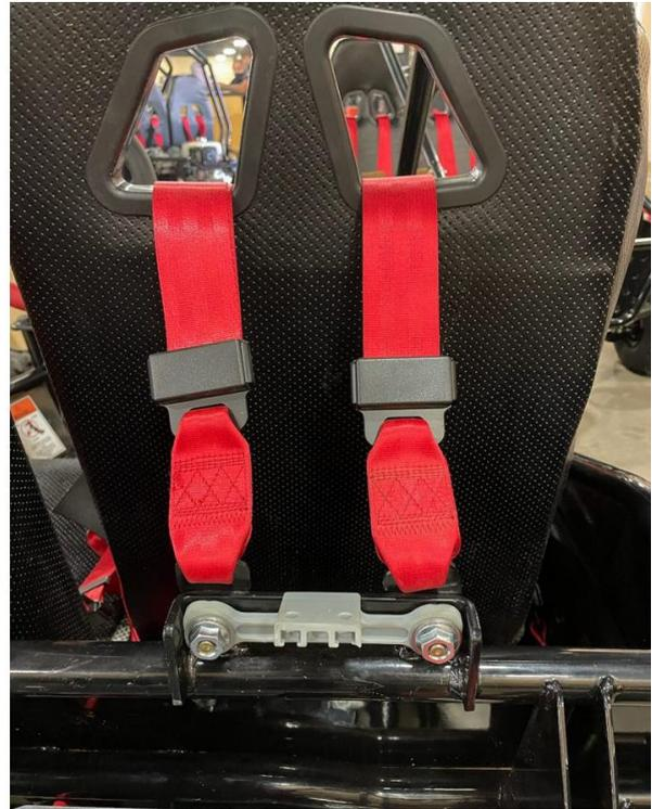
Image: 3D-printed go-kart parts printed with engineering 3d resins: Strong-X and Tough-X resin for the Torque Off Road TQ390.
