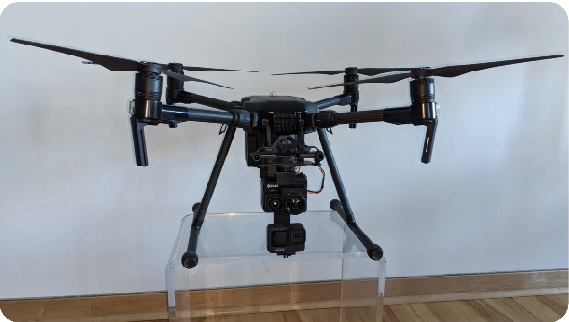
Part of the Dragontech platform incorporates the LIDAR, Multi-Spectral Spectral Sensors, and a controller attached to an enterprise drone via mounts 3D printed on the MakerBot METHOD X using Nylon Carbon Fiber.
