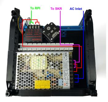
Install the AC inlet and complete the wiring of the power supplies, the end result should look something similar to this:
