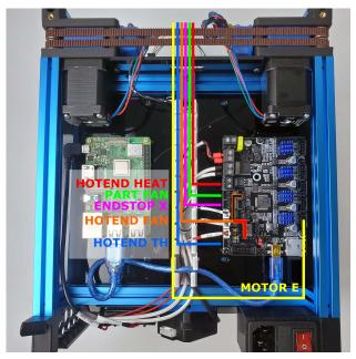
Be especially careful with the hotend fan connection, as it is easy to insert either pin into the wrong place (double check with the manual). The end result should look like this:
