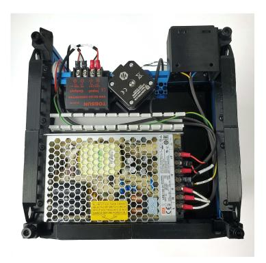
Finally, cover up the PVC duct and PSU.
