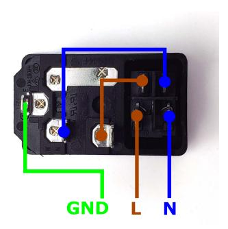
Take the inlet cable included in the kit and attach the wires using the above layout as reference. When wired correctly, your live wire will be protected by a fuse, and the switch on the front side of the inlet will operate correctly (lights up when turned on).
