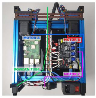
After connecting all the wires, you can now cover up the PVC duct. Wiring is now complete!
