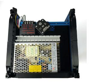
Use VHB tape to stick the PVC duct onto the bottom panel
