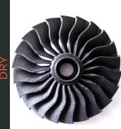
The turbine blade on the left was printed with wet Covestro Addigy® F1030 CF10 filament, while the one on the right was printed with Drywised filament. The image clearly shows that all the oozing and stringing has rendered the print unusable. Furthermore, the inconsistent extrusion has caused the thin walls of the part to have inferior strength.
