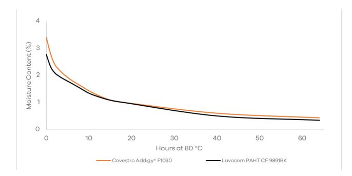
From the figure above, it can be observed that it takes at least 40 hours of drying to reduce the moisture content of 3.4% Covestro Addigy<sup>®</sup> F1030 (2.85 mm) filament to around 0.5%. A level which is acceptable for printing. A further 24 hours are then needed to reduce it to 0.43%. It can also be observed that while the filament loses a lot of moisture initially, the rate of moisture loss slows down as it loses more moisture.
