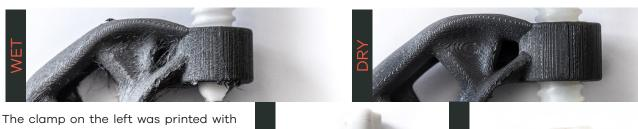
The clamp on the left was printed with wet Jabil PA0600 (gray) and Covestro Addigy® F1030 (natural) filaments. The filament used for the clamp on the right were Drywised. Apart from the visual imperfections, the clamp which was not dried could not be screwed in due to the variation in tolerances brought about by the presence of moisture in the material during printing.
