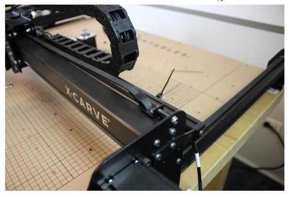
(Left side of belt is not show, attach using smaller button head capscrew)
