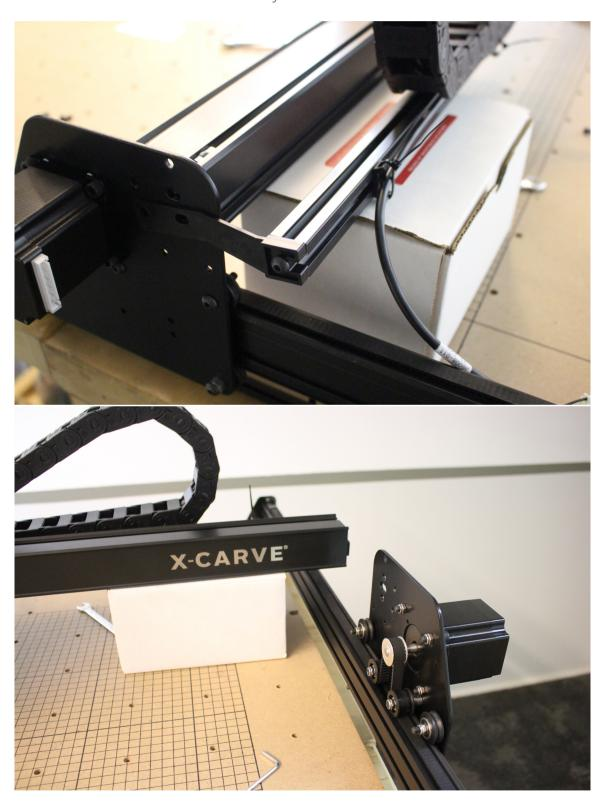
Carefully slide the x-carriage off of the wide makerlide. You may need to <u>adjust</u> the eccentric spacer to the open position to allow the x-carraige to move easily.
