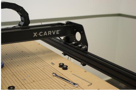
For each idler, you'll use the existing screw, spacer and locknut plus 2 M5 washers and the 9mm idler.
