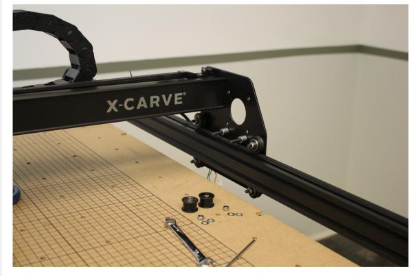
The order of assembly is as follows: screw through plate, spacer, idler, two M5 washers and locknut. Make sure the idler is positioned correctly with the inset part facing out away from the screw head.
