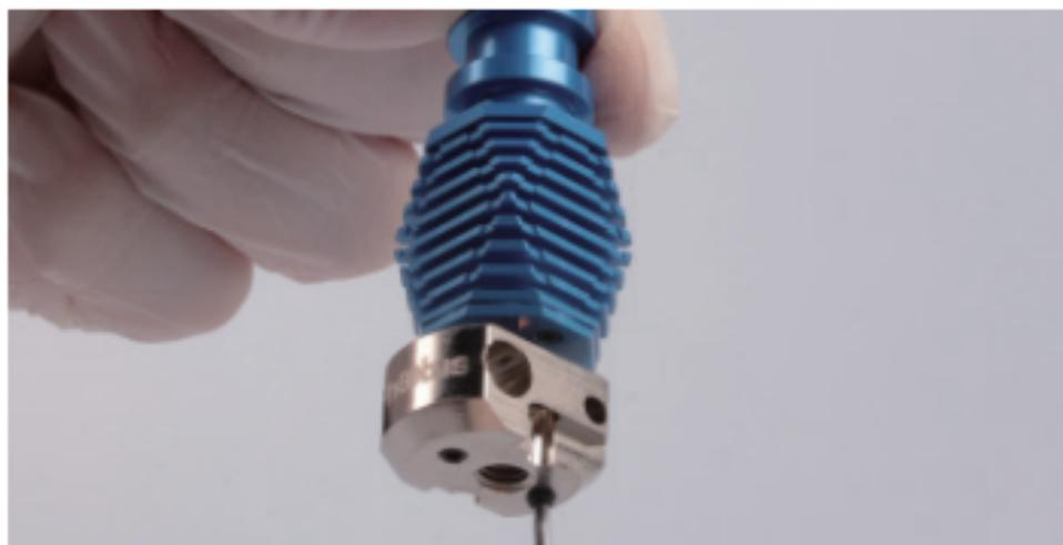
8. Put the silicone sock onto the heat block.
