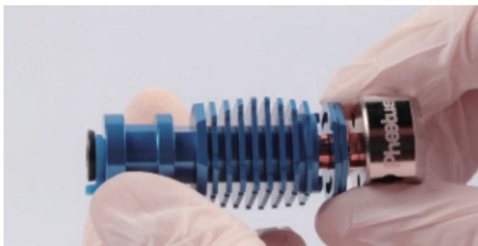
6. Put two M1.4 screws into the rib and use 1.27 hexagonal bar for locking.
