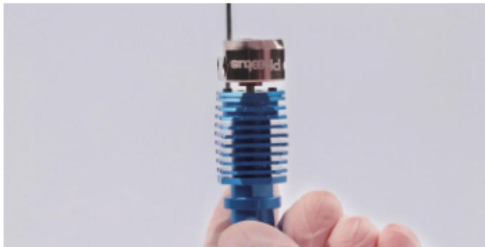
7. Screw two M3 head screws into the correct holes on the B - side of the heat block respectively by using 1.5 hexagonal bar.
