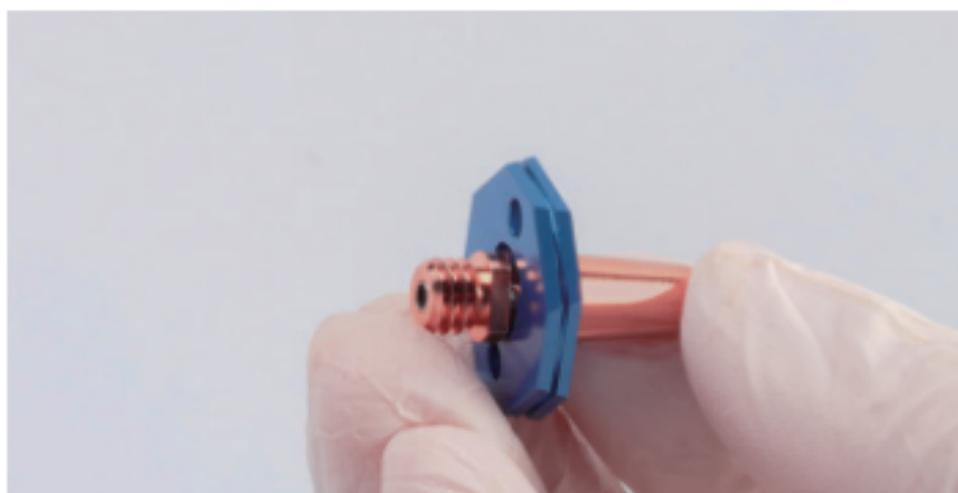
4. Screw the heat break into the side - A of heat block by using 5mm open - ended wrench (Attention: Side - A of heat block should be completely attached to the heat break).
