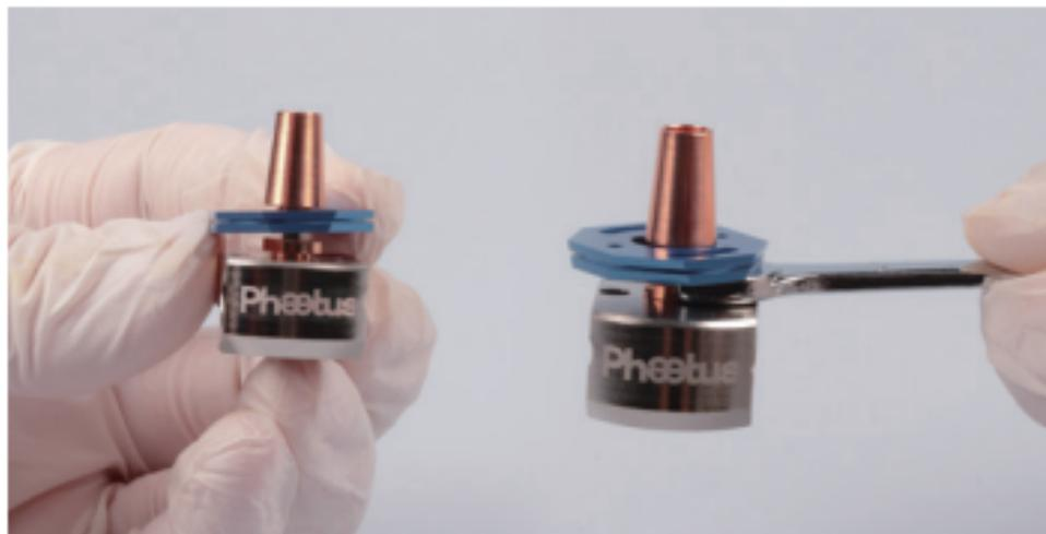
5. Assemble the heat break into the heat sink and adjust its position, so that the side plane of the heat sink, which close to its threaded hole, and the 2 through holes on the heat block, are align with the 2 holes on the heat sink.
